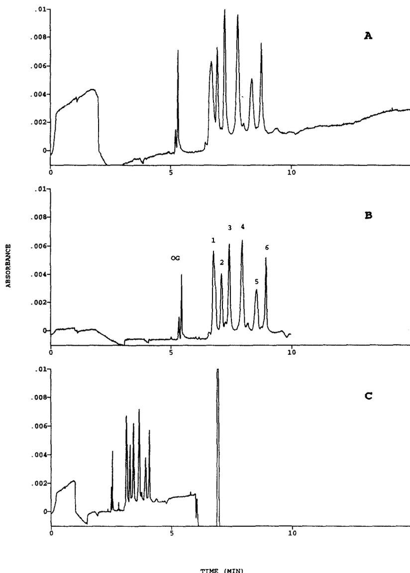
Fig. 1. The effect of capillary diameter on the separation of standard proteins using eCAP SDS 14-200 kit. (A) 27 cm  $\times$  100  $\mu$ m I.D. capillary; 300 V/cm field strength; 5-s pressure injection; (B) 27 cm  $\times$  50  $\mu$ m I.D. capillary; 300 V/cm field strength; 20-s pressure injection; (C) 27 cm  $\times$  50  $\mu$ m I.D. capillary; 633 V/cm field strength; 20-s pressure injection. Peaks: OG = orange G; 1 = ALACT; 2 = STI; 3 = CA; 4 = OVAL; 5 = BSA; 6 = PHB.
