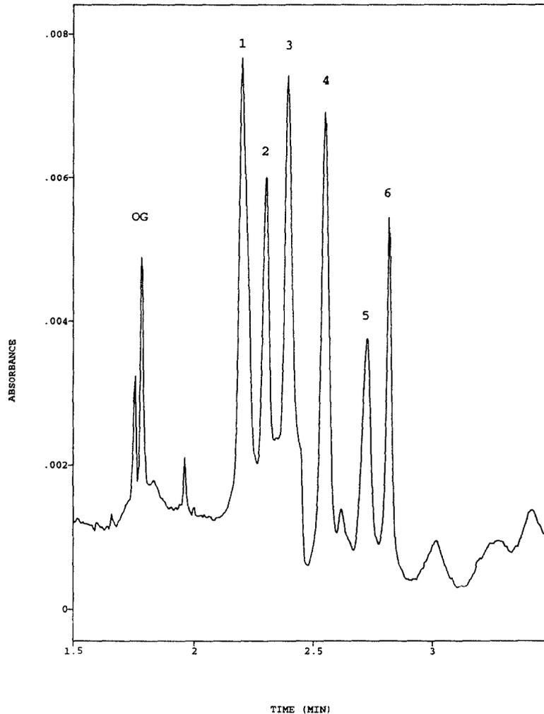
Fig. 2. Separation of standard proteins at high field strength. Capillary dimensions;  $27 \text{ cm} \times 50 \text{ }\mu\text{m}$  I.D. Electrophoresis conditions:  $888 \text{ V/cm}$  field strength and 20-s pressure injection. Peaks as in Fig. 1.
