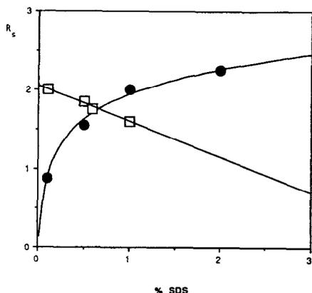
Fig. 3. Effect of the SDS concentration in the separation buffer (□) and in the sample buffer (●) on the resolution between the  $\alpha$ -lactalbumin and carbonic anhydrase peaks.
